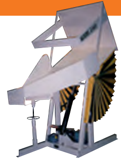
STATIONARY DUMPER WITH ADJUSTABLE CHUTE ATTACHMENT AND SAFETY SKIRTING
